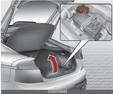
Battery box fuse pane
