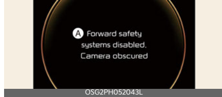
A: Forward safety systems disabled. Camera obscured
