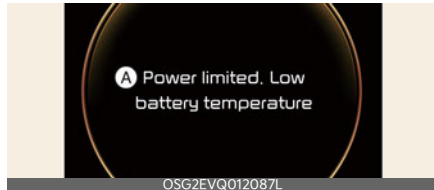
A: Power limited. Low battery temperature
