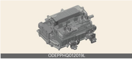
High voltage battery system *2
