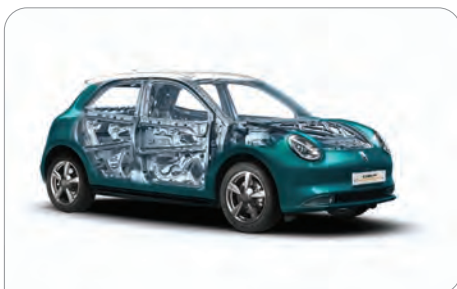
Iron Bone - Ultra-high Strength Steel Body Frame
