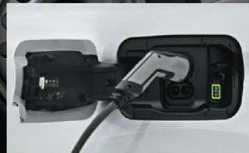
GREEN DIODE WHEN CHARGING IS COMPLETE
