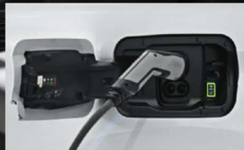
FLASHING GREEN DIODE FOR CHARGING IN PROGRESS
