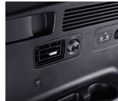
3rd Row Air Conditioning System
