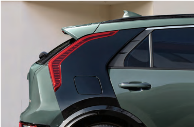
C-pillar aero duct The C-pillar design highlights the profile of the car. To prevent static pressure, the aero-pillar has an opening to let airflow through.
