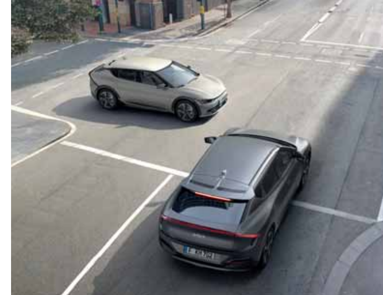
Forward Collision-Avoidance Assist with junction turning and crossing (FCA). FCA uses a front-view camera and radar to detect any vehicles, pedestrians or cyclists ahead. By warning and braking automatically, it can help you avoid, or reduce the severity of, an accident. The system also engages if you are crossing or turning at an intersection.
