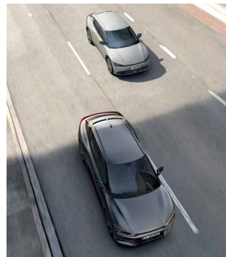
Blind-Spot Collision-Avoidance Assist (BCA). When you signal a lane change, you will be warned if a risk of collision with a vehicle approaching from the rear is detected. If the risk persists and increases, BCA automatically controls the vehicle to help avoid a collision. If you are exiting a parallel parking spot and there is a risk of a collision with an approaching vehicle, BCA automatically applies emergency braking.
