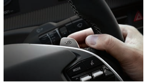
Smart regenerative braking system (SRS 2.0)
