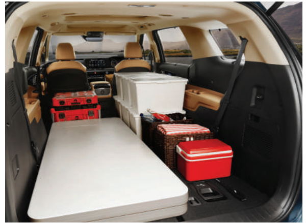
Luggage mode For 7- or 8-seater models, a lever lets you fold down the 3 rd row seat to accommodate more boot space. Expand your luggage space from 627ℓ to 2,905ℓ with only the first row of seats in use.
