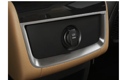
Center-console power outlet
