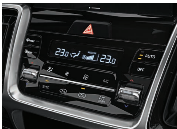
Dual-zone full auto air conditioning system and 3rd row rear air conditioning system
